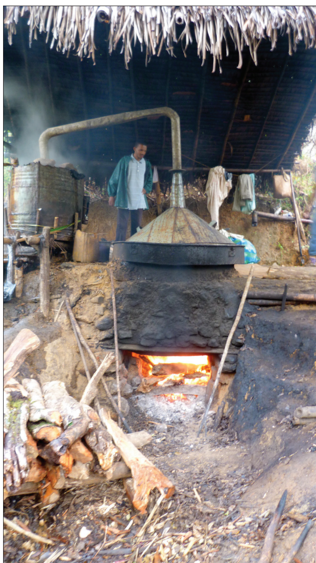
FIGURE 3. A wood-fired still producing clove essential oil in the area of Fénériver-Est, Region Analanjirofo, Madagascar. Notice the bare fire and the dilapidation of the equipment, which results in low yield and an important volume of wood used per batch of distillation, which has more often become fruit trees (mango tree, lychee tree, breadfruit trees or old clove trees). Photo E. Penot.
