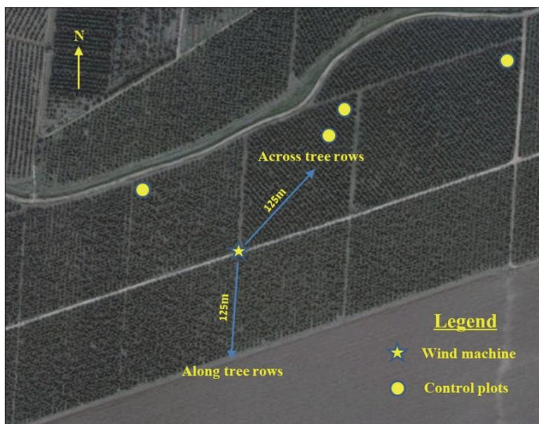
**FIGURE 1.** Satellite image of the experimental avocado orchard. The locations of the wind machine, the control plots, and the two measured sectors are marked with a star, circles, and arrows, respectively.
