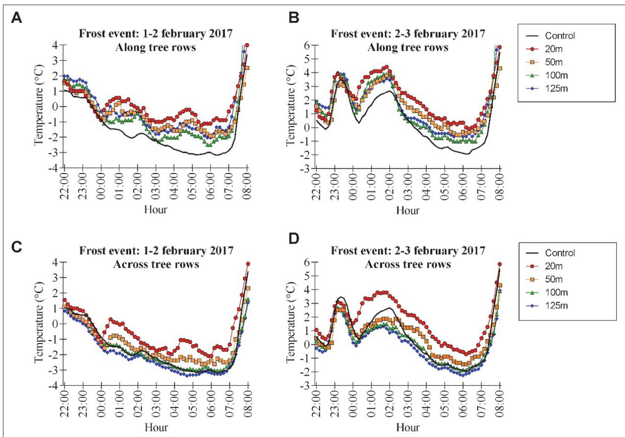
**FIGURE 3.** Night-time air temperature at 1.5 m above ground 20, 50, 100, and 125 m from the wind machine. A, B: parallel to the tree row on 1<sup>st</sup> to 2<sup>nd</sup>, and 2<sup>nd</sup> to 3<sup>rd</sup> of February, respectively. C, D: across the tree rows on 1<sup>st</sup> to 2<sup>nd</sup>, and 2<sup>nd</sup> to 3<sup>rd</sup> of February, respectively.
