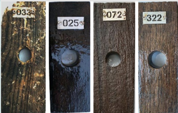
033: Scots pine ( Pinus sylvestris ) after 1 year 025: Acaria ( Minquartia guianensis ) after 22 years 072: Azobe/Ekki ( Lophira alata ) after 8 years 322: Angélique ( Dicorynia guianensis ) after 6 years
