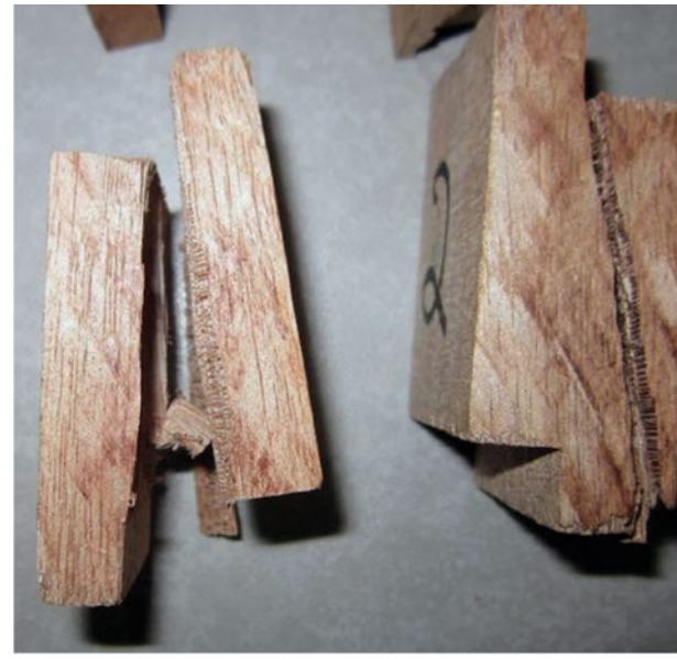
Figure 3. Post-test image of two specimens of Abura ( Mitragyna ciliata ) wood.
