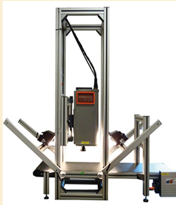
Photo 1. Near-infrared (NIR) hyperspectral imaging system (courtesy of the Walloon Agricultural Research Center, Belgium). Photo N. Kayoka Mukendi.
