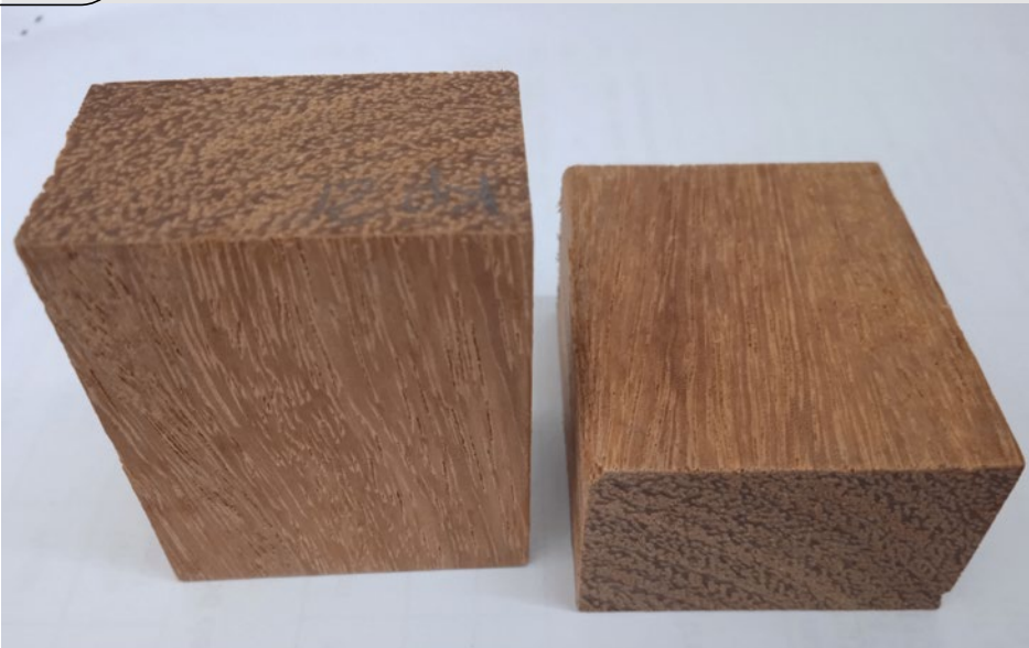
Photo 2. Two test blocks {2.5 × 4 × 5 (length) cm} of kempas ( Koompassia malaccensis ) heartwood representing structural medium density hardwoods used in Malaysia. Photo A. H. H. Wong.
