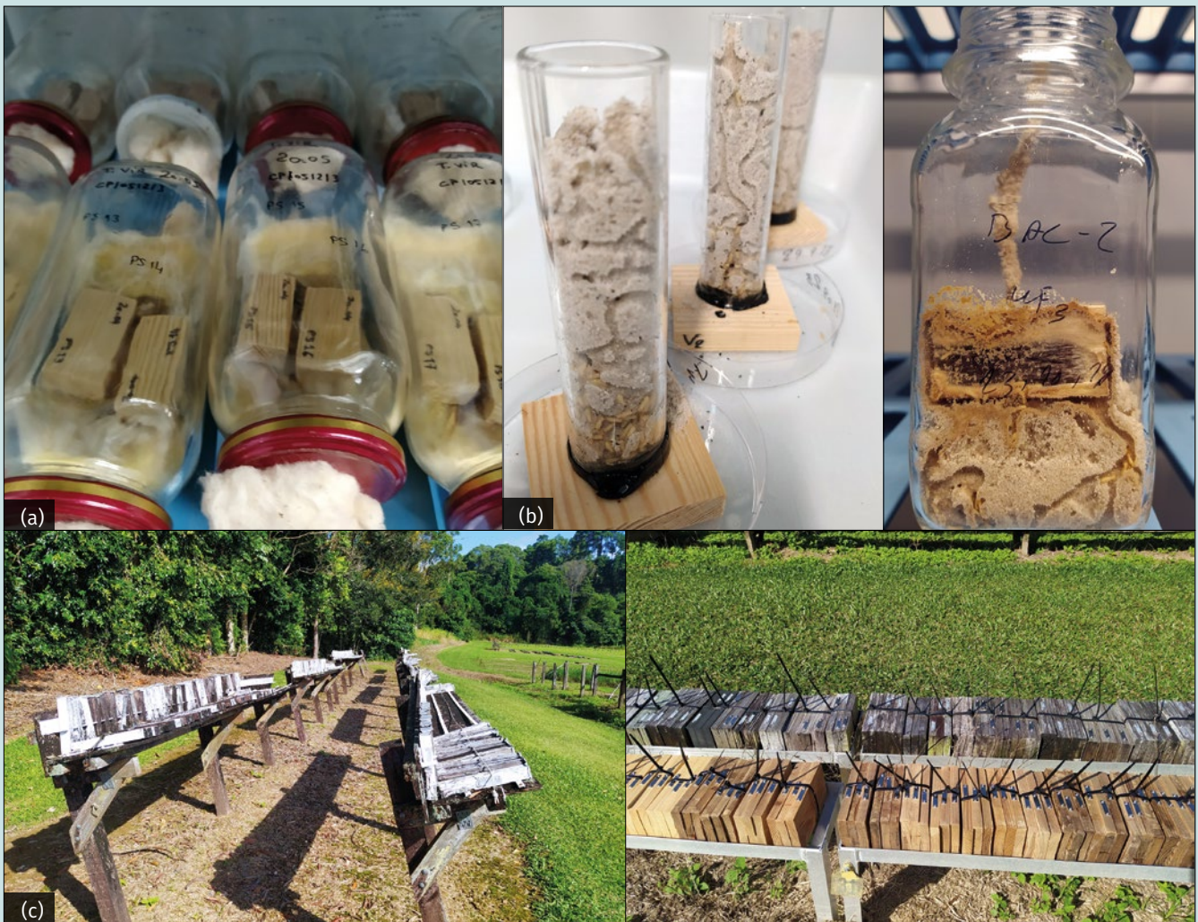
Figure 2. (a) Examples of fungal decay test in French laboratory (EN 350-2). (b) Termite resistance test in French laboratory (EN 118 and EN 117). (c) Field tests in Queensland - Australia. Photos © K. Candelier.
