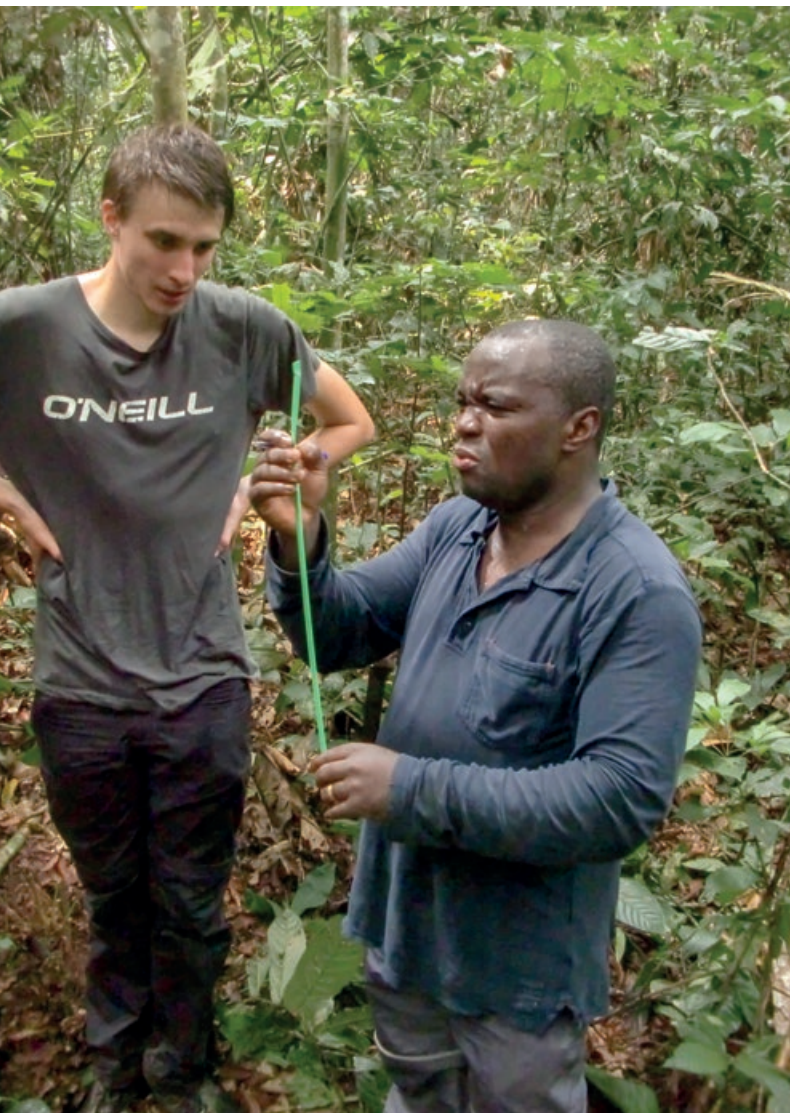
Photo 3. Sampling straw used to record data from a core extracted from a stem of Entandrophragma sp. in the buffer zone of the Yangambi Biosphere Reserve. Photo M. Devriendt.
