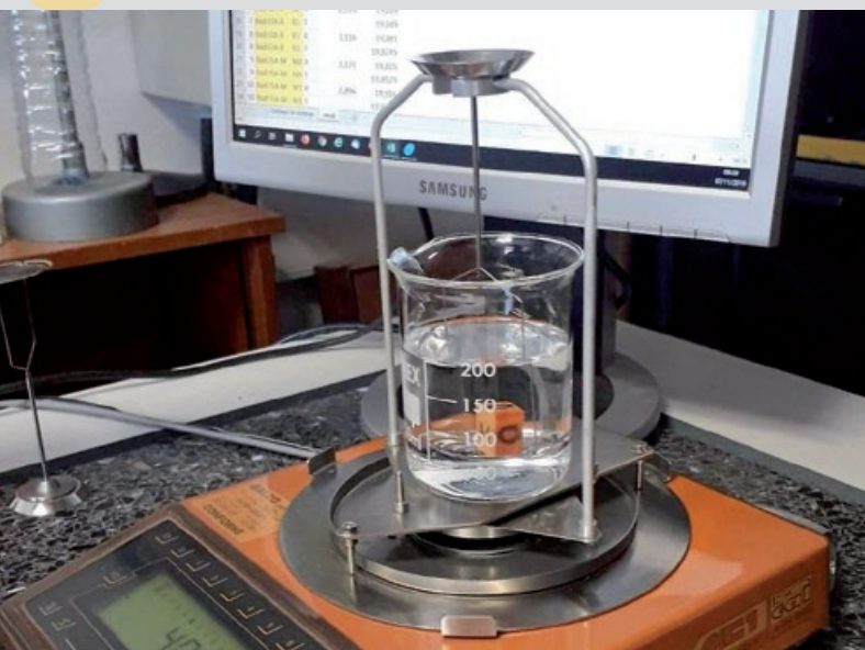
Photo 4. Balance Sartorius. Sartorius scale device. Photo D. Dougabka.
