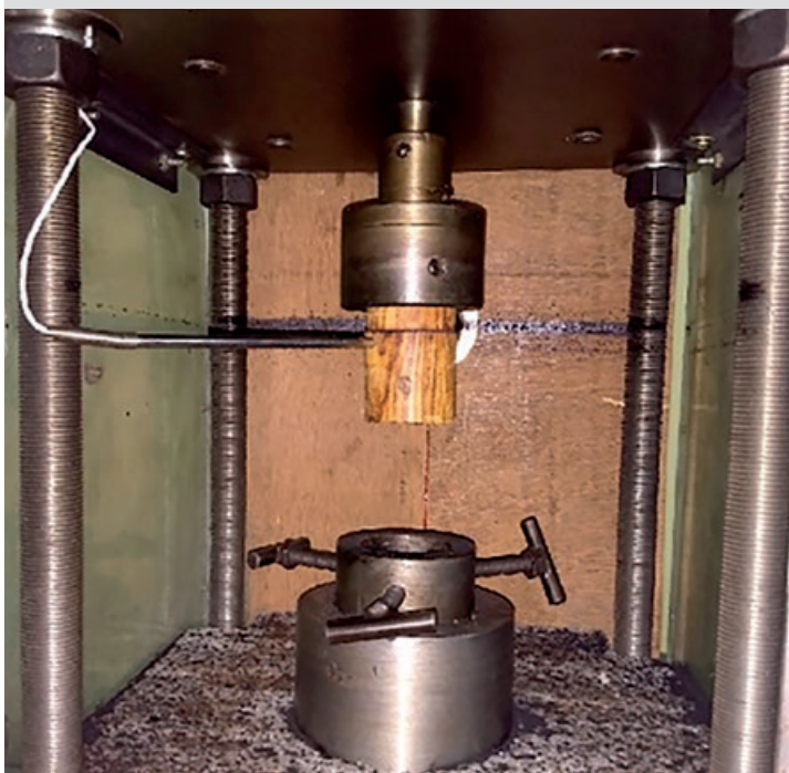
Photo 3. Recording weld line temperature using PT-100 type thermo-couple.
