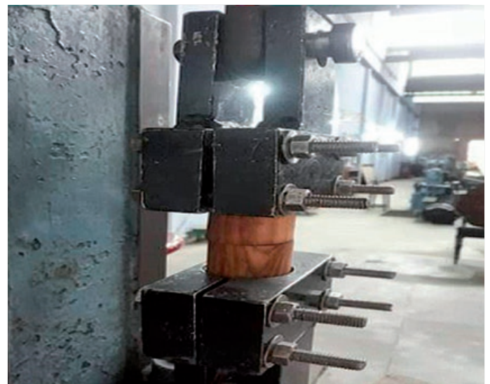
Photo 4. Tensile strength testing.
