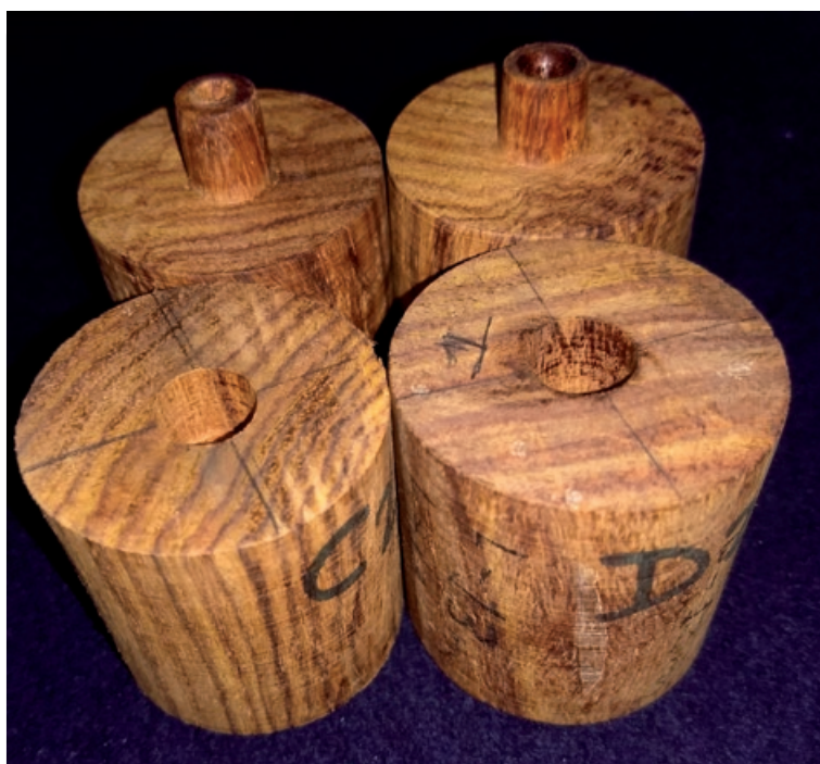
Photo 2. Tongue-and-groove wood welding samples.
