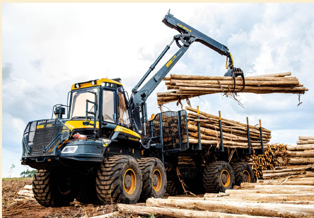
Photo 1. Forestry forwarder used to extract round timber from a eucalyptus plantation in southern Bahia, Northeastern Brazil. Photo C. F. Lima.
