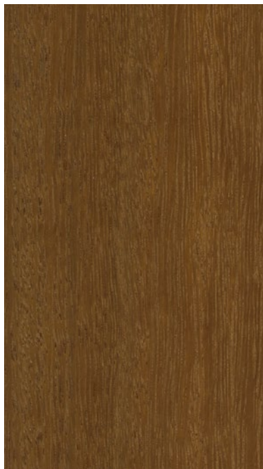
Half-quarter sawn. Photo D. Guibal, Cirad.
