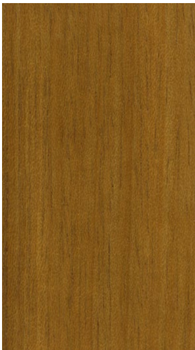
Half-quarter sawn. Photo D. Guibal, Cirad.
