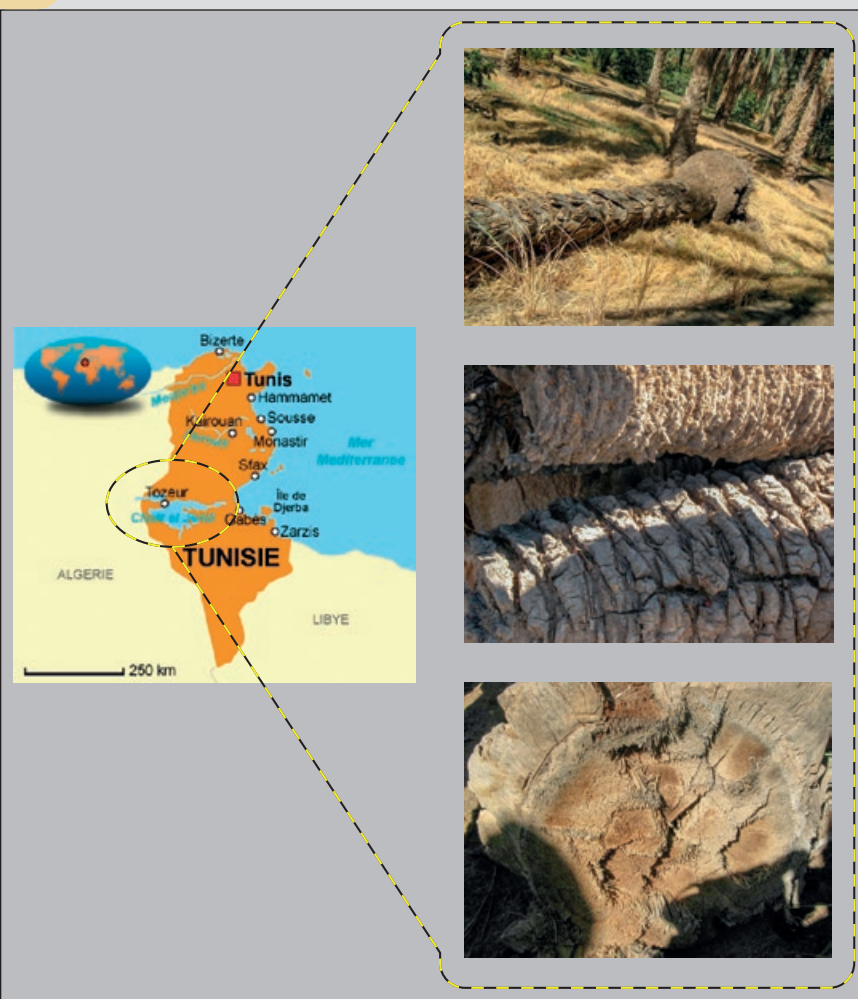
Figure 3. Exposition of date palm tree trunk, freshly slaughtered, into the salt waters cycles into the Lake of Chot Djérid.
