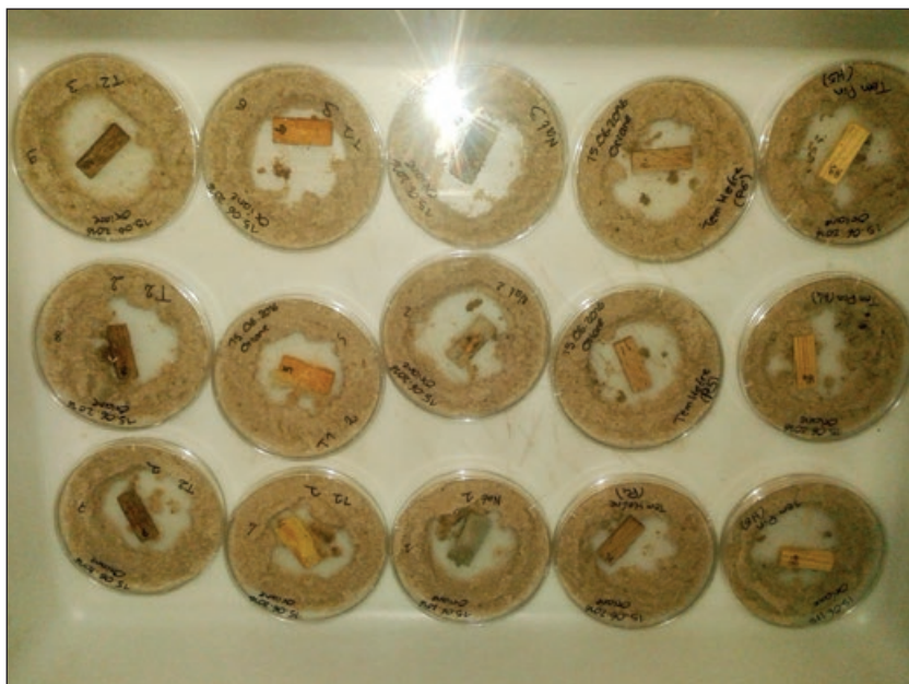
Figure 5. Screening termites test devices, with adjustments to EN 117 standard guidelines, for beech and pine wood controls and date palm woods.
