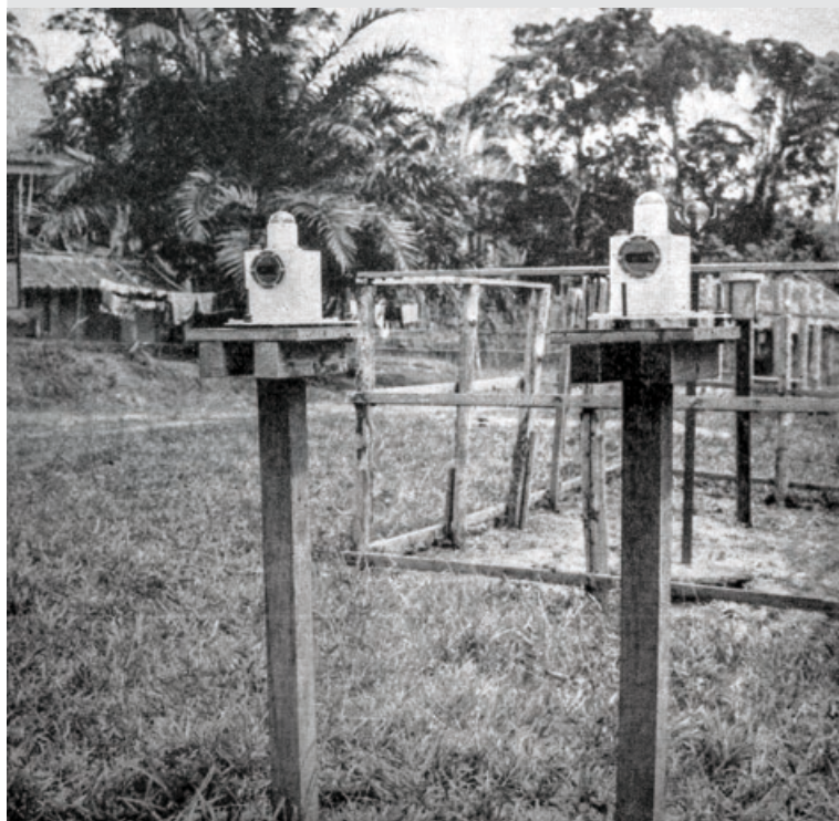
Photo 2. C.T.F.T., Gabon. Ikoy-Bandja Forestry Station. A pair of prototype Borrel solar meters set up on open ground to check their operation. Note their robust appearance. Photo Leroy-Deval.
