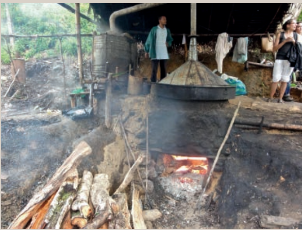
Photo 6. Still used for clove oil distillation at Sainte-Marie (November 2011). Photograph P. Danthu.
