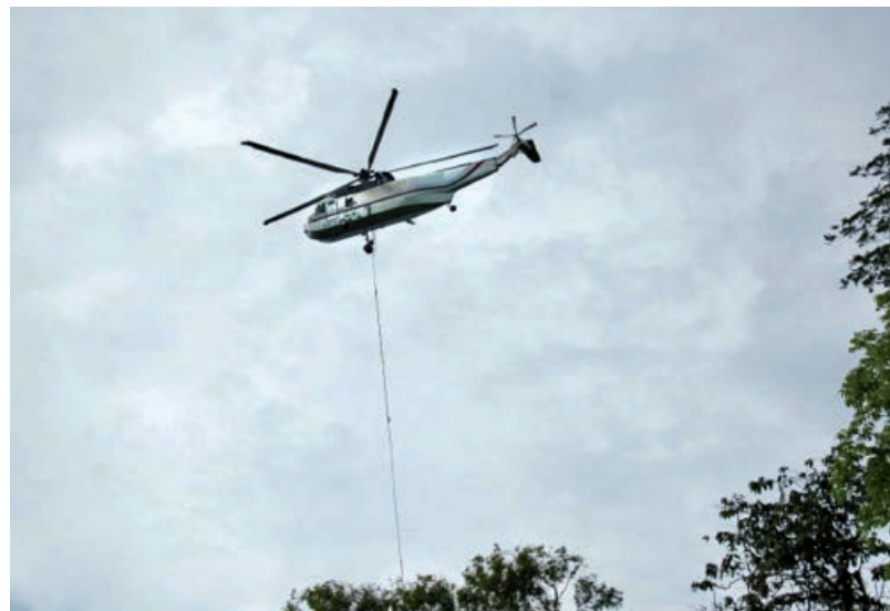
Photograph 2. Low-impact logging system using helicopter. Photograph H. Bigsby.
