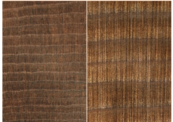
Photos 7. Alerce ( Fitzroya cupressoides , CITES Annex I, left) and Western Red Cedar ( Thuja plicata , right) are virtually indistinguishable given their similar structure. The aromatic odour and yellowish hue of Western Red Cedar, however, is of much help in distinguishing between the two timbers. Photos C. Waitkus (vTI).
