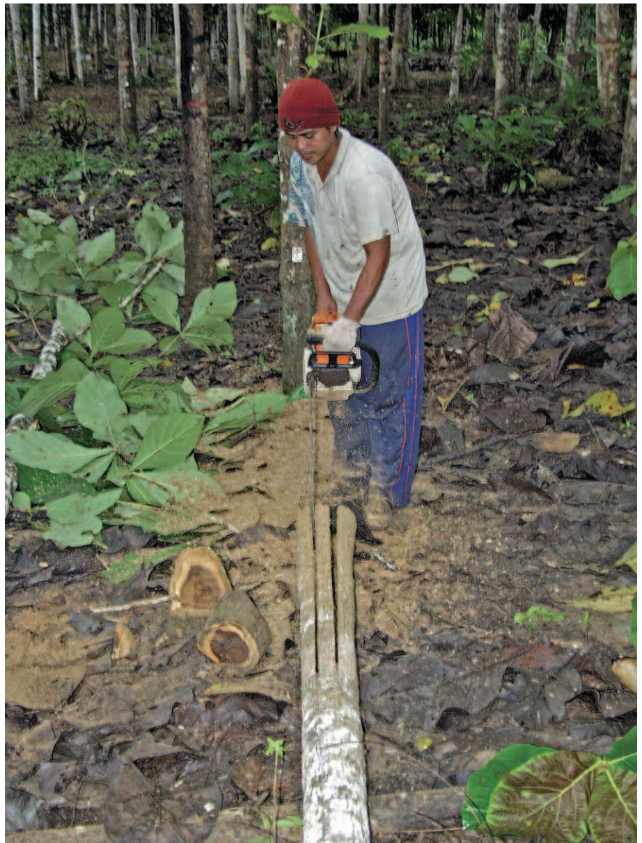
Photo 2. Board destructive sampling using a chainsaw. Photo O. Monteuis.
