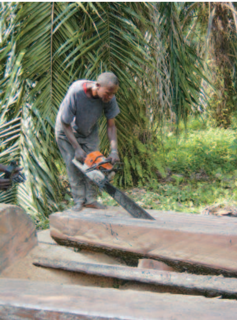
Freehand chainsaw milling in the Democratic Republic of Congo. Photo C. Fehr.
