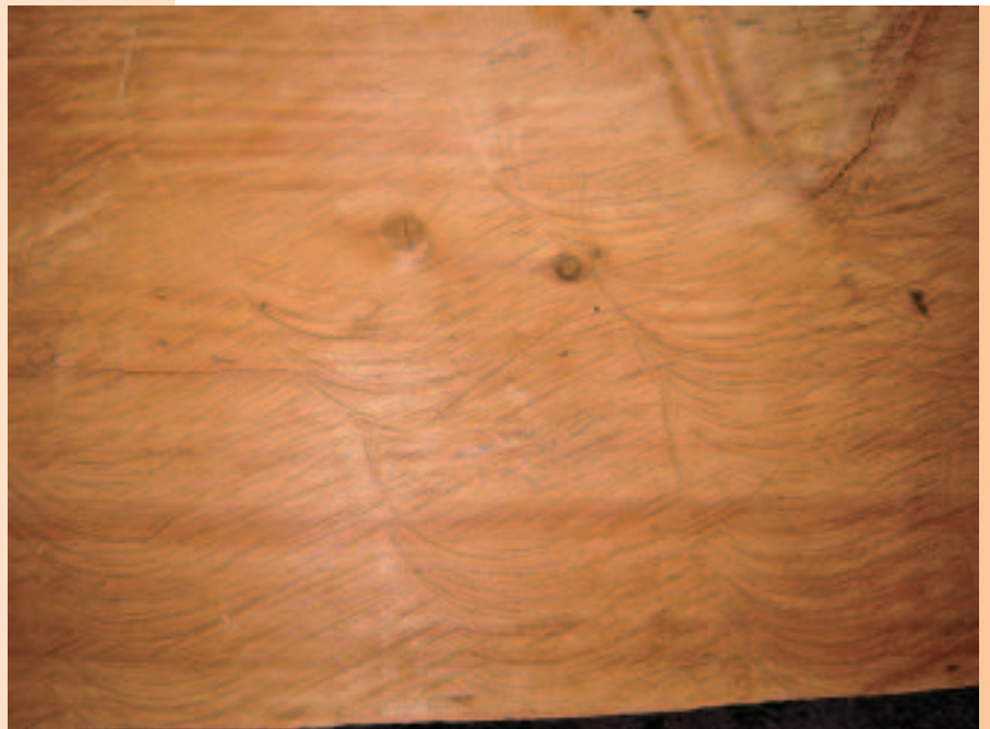
The tell-tale “trademark” of chainsaw milled timber on mahogany ( Khaya spp.) from the Democratic Republic of Congo as seen in Nairobi, Kenya. Photo N. Pasiecznik.
