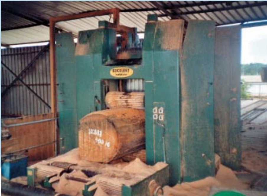
Scie battante multilame. Multi-bladed stock saw. Photo C. Daigremont.
