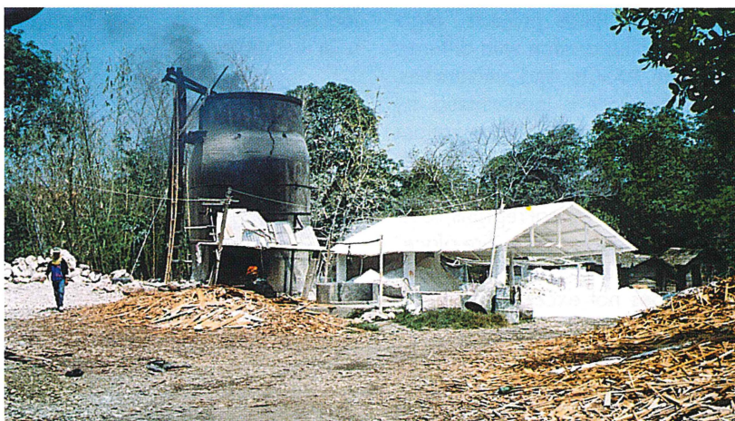
Small-scale production of lime in Indonesia using sawmill waste.
