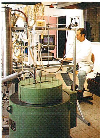
The CIRAD-Forêt carbonization laboratory in Montpellier : an experimental retort with its waste recovery system.
