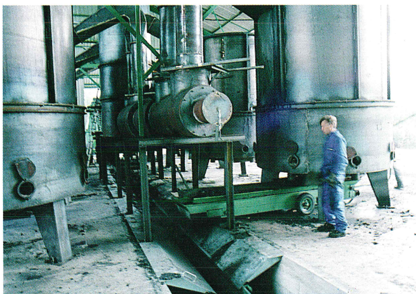
Carbonization exhaust gas treatment system by incineration (CML process).
