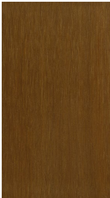
Flat sawn. Photo D. Guibal, Cirad.
