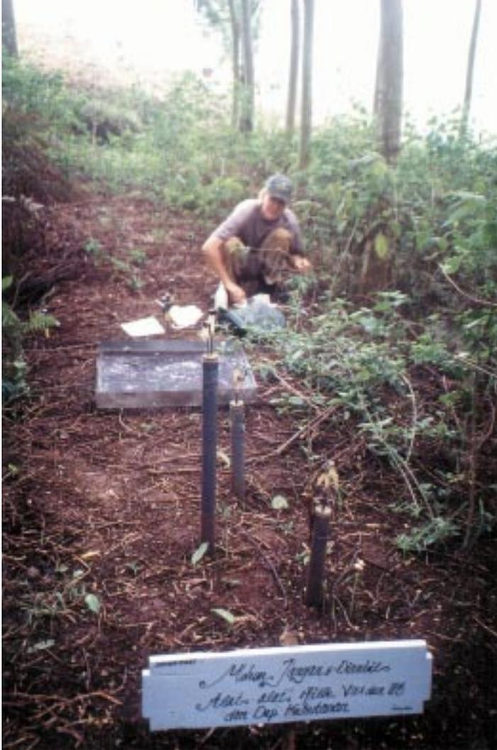
Setup to measure components of the forest carbon cycle (from front to back): vacuum tube lysimeters to sample soil moisture, a leaf litter trap, tensiometers to measure soil water suction, and researcher R.R.E. Vernimmen.
