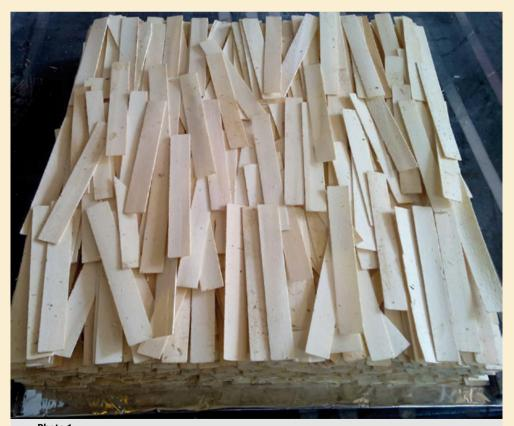
**Photo 1.** Oriented strand lumbers (OSL) mat before being placed in the hot-press. Photo H. R. Taghiyari.
