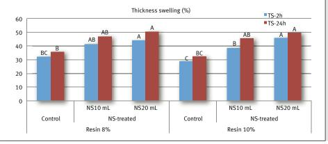
Figure 4. Water absorption and thickness swelling values in the six oriented strand lumbers (OSL) panels produced (NS=nano-silane content).
