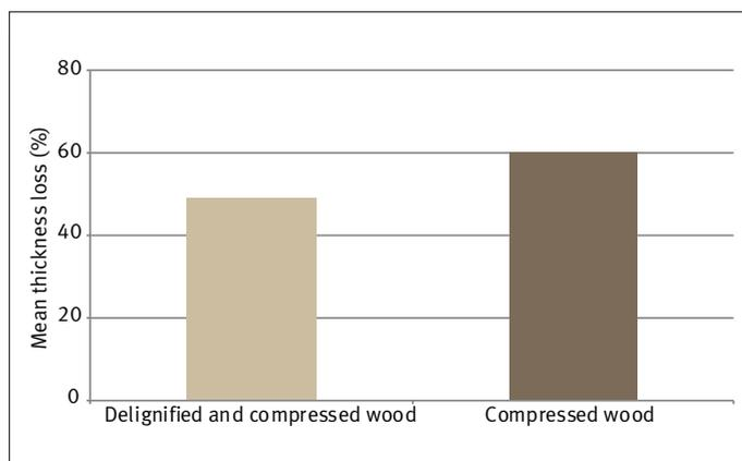
**Figure 4.** Thickness loss in sample with delignification and without delignification.
