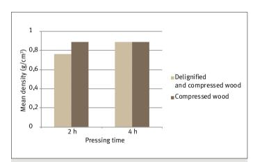
**Figure 3.** Effect of pressing time of wood density.
