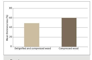
**Figure 4.** Thickness loss in sample with delignification and without delignification.
