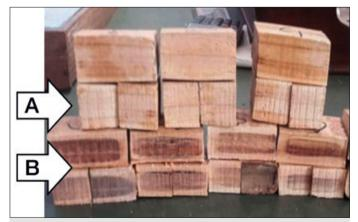
Figure 1. Compressed wood specimens: A. Compressed without delignification (CW). B. Delignified and compressed.
