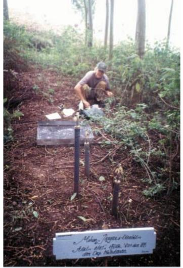
Setup to measure components of the forest carbon cycle (from front to back): vacuum tube lysimeters to sample soil moisture, a leaf litter trap, tensiometers to measure soil water suction, and researcher R.R.E. Vernimmen. Photo A.I.J.M. van Dijk.
